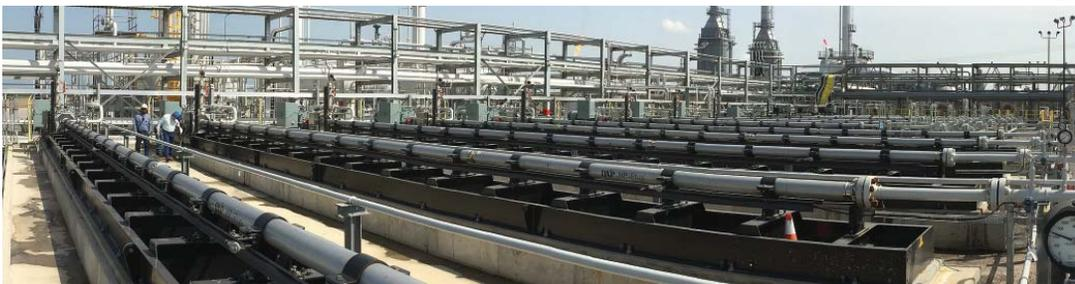
The PumpWorks HP-Plus pump was designed with reliability and cost reduction in mind. It is a multi-stage centrifugal pump capable of producing a full range of volumes and pressures. Each pump is individually assembled by trained PumpWorks personnel and fully tested to industry API 11S2 standards.
