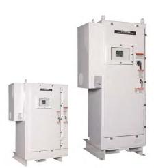
protection. The Plus Pack is a solid-state AC drive that ranges from 66-1500 KVA and features true torque control enabling motors to develop high starting torque and compensating for motor slip. Available in NEMA 3R enclosures, ASD rated for 50 degrees C and 4500 fasl with no derate of output current. The enclosure cooling
